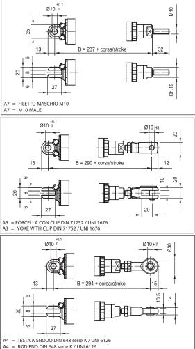
**Note:** "B" dimension changes according to model Note: With encoder, dimension "B" is 30 mm longer L02 = See pictures L02 stroke > 320 mm = + 11 mm L02-FCM = +34 mmL02-FCM stroke > 320 mm = +45 mmwith safety nut "G'' = +30 mmL02-VRS = +40 mmBellows + 20mm (no for versions FCM)
